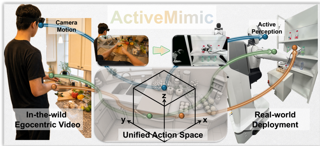
Figure 1: ActiveMimic acquires active perception from in-the-wild egocentric human video and transfers it to real-world humanoid robots. Left to center : egocentric camera motion and wrist action together form a 27-dimensional unified action representation that enables the model to jointly learn active perception and manipulation. Center to right : active perception is transferred to a humanoid robot, which repositions its viewpoint actively during task execution.
