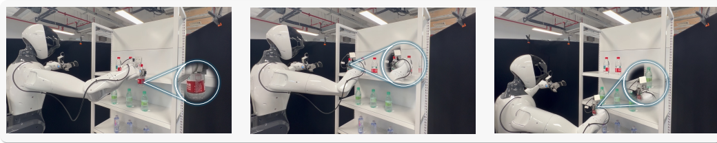
Figure 10: Representative failure cases of ActiveMimic without the head camera on Restocking. All three failures occur at the placement point. From left to right: (1) correct shelf tier and lateral position, but the placement motion is imprecise and knocks over the shelf; (2) correct tier, wrong lateral position; (3) wrong tier entirely. All three stem from severing the visual loop that the pretrained model relies on to coordinate head and hand movements during active perception.
